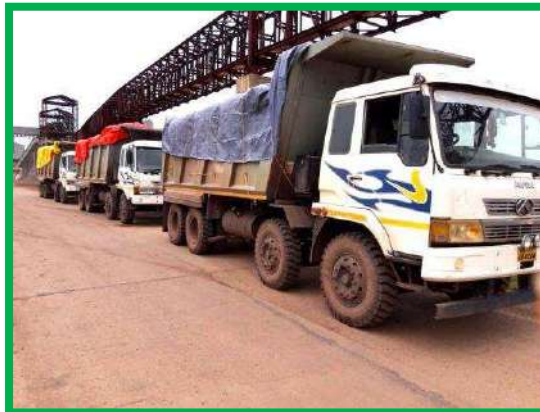
Tarpaulin covered trucks for transporting Raw materials from Limestone mines
